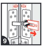
Remove the retaining plate. Ensure that it is kept in a safe place in case it is necessary to remove the closer from the door at any time.
