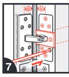
Insert the body of the closer into the door leaf, with the retaining plate facing you, and screw fix.
