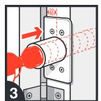
Drill the hole for the closer body using the Lewis auger bit.
