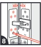
Fix the plate onto the door frame making sure it is exactly in line with the other plate.
