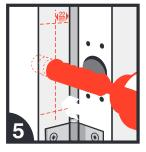
Drill out a centre hole 15mm diameter to a depth of 10mm.
